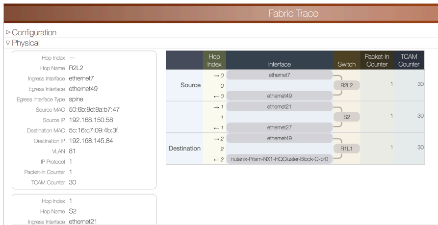
Figure: Fabric Trace showing hop-by-hop physical connectivity for Nutanix VMs in Big Cloud Fabric
