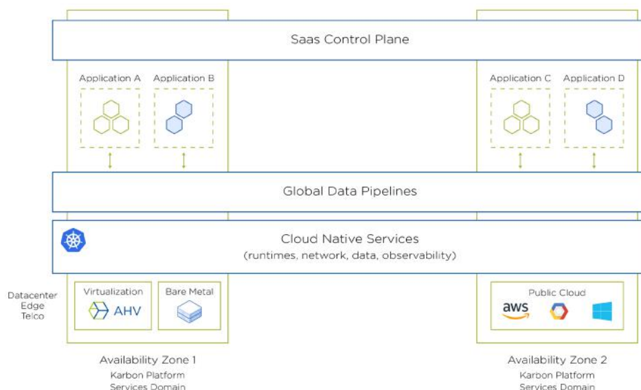
FIGURE 1: Karbon Platform Services Architecture
