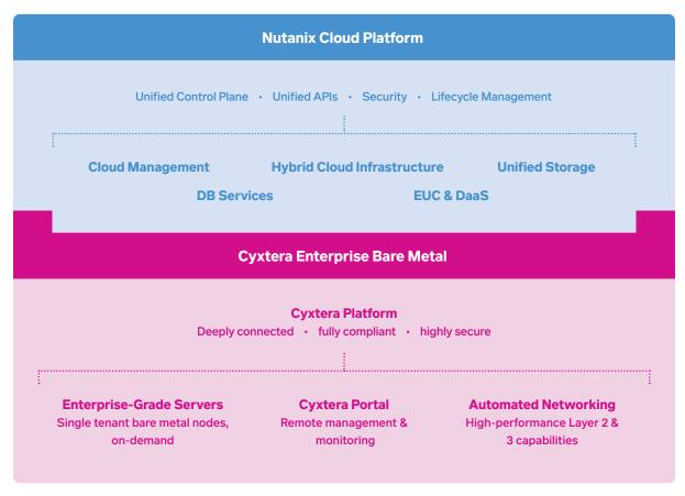
When creating the Nutanix/Cyxtera technology stack, Enterprise Bare Metal forms the foundation for the Nutanix solution.
