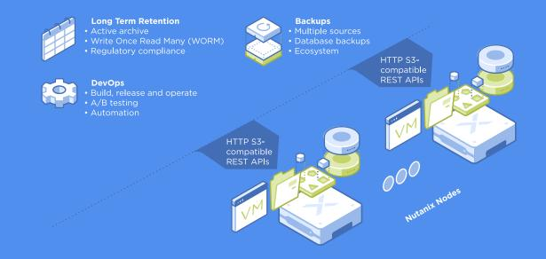
Objects is implemented using scale-out Object Volume Managers (OVMs) each running on a separate cluster node. This architecture allows seamless performance scaling either by adding more OVMs, or by increasing the CPU and memory resources allocated to each OVM.
